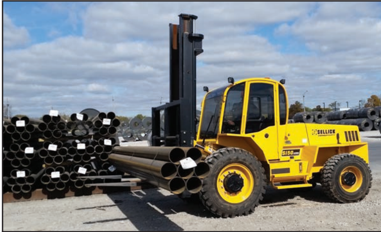
2 and 3 stage heavy duty all roller masts are designed for high duty cycles with little maintenance required
