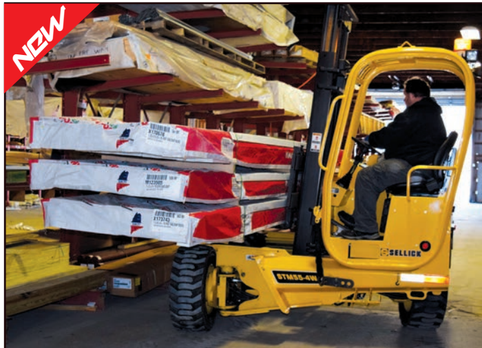
With the press of a button, the STM55-4W transitions for sideways operation
