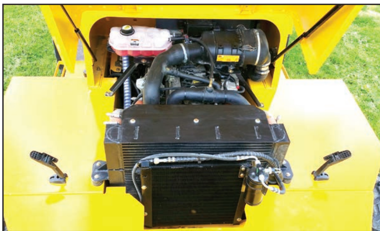
Tier 4 Ecomax engine provides high torque with no exhaust aftertreatment or fluids required.
